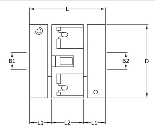
$\begin{array}{lll} B1 & = 5 \\ B2 & = 6 \\ D & = 27 \\ L & = 25.4 \\ L1 & = 9.3 \\ L2 & = 6.9 \\ Screw = M3 \end{array}$
